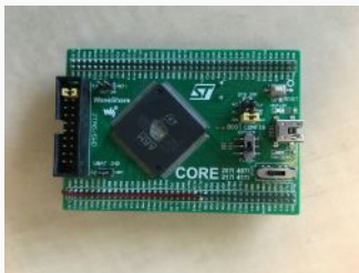
Figure: Modified Pinata ARM STM32F417IG device.
